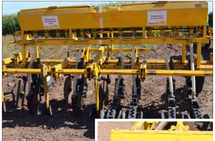
Sowing machine for planting wheat on two rows/bed ...
