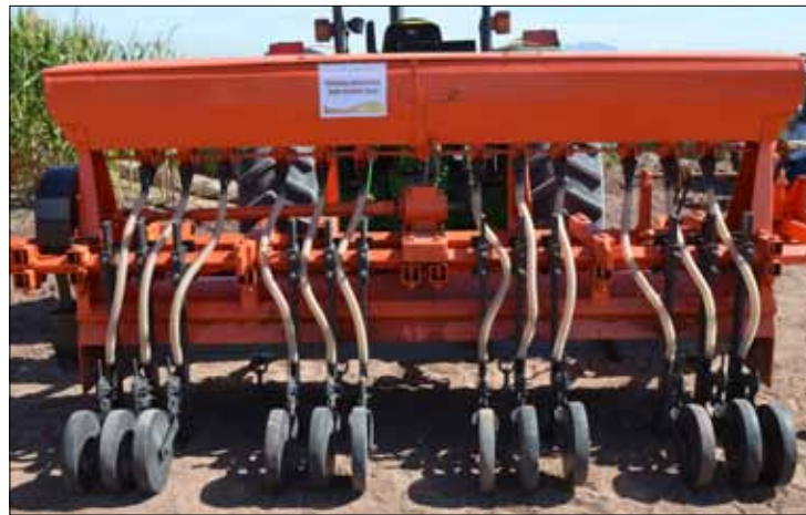
Sowing machine for planting wheat on two rows/bed ...
