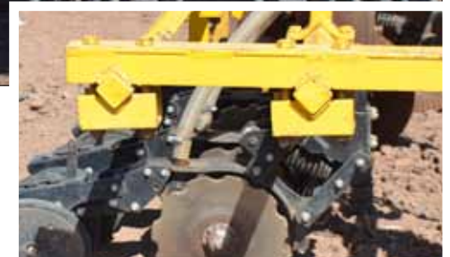
... featuring scalloped, twin disc openers and twin press wheels.
