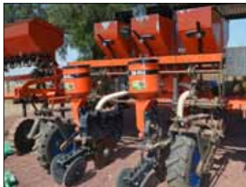
A multi-use seeder and fertiliser machine for small grains set up with bed formers and sowing tines.
