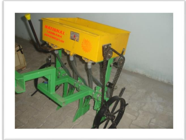
A basic National seeder from the Punjab. It can seed a range of crops on all soil types, and can place fertiliser with the seed
