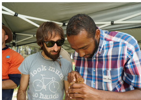
Student ambassadors are shown how to carefully inspect the core faces to count the crop roots and to compile the data for analysis.
