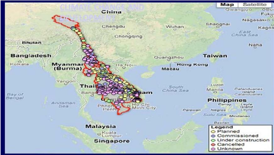
Figure 5. Types of barriers across the Mekong Basin: planned, commissioned, under construction, cancelled, unknown (see legend). *Source:* CGIAR.
