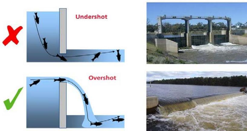
**Figure 14.** More fish survive overshot weirs (lower diagram & photo) compared to undershot weirs (upper diagram & photo).
