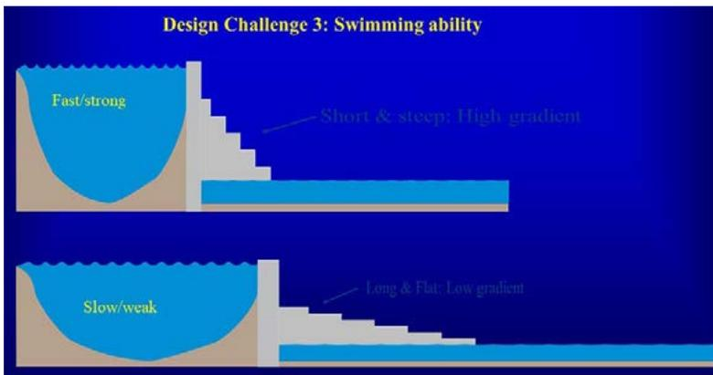
Figure 11. Differing swimming abilities need to be accommodated.
